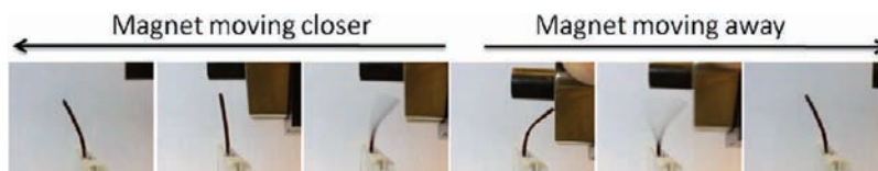
Figure 11. Actuation of LC ferrogel 116 using a magnet.
